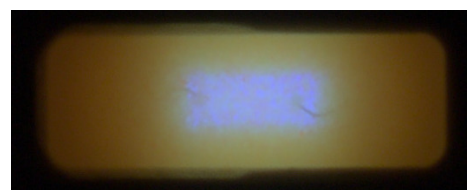
Closeup of a 4014 LED chip
